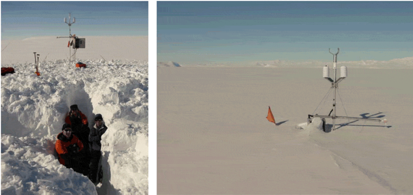
Fig.1: Automatic weather station at Skinner Saddle after excavation (left image) and before (right image)
