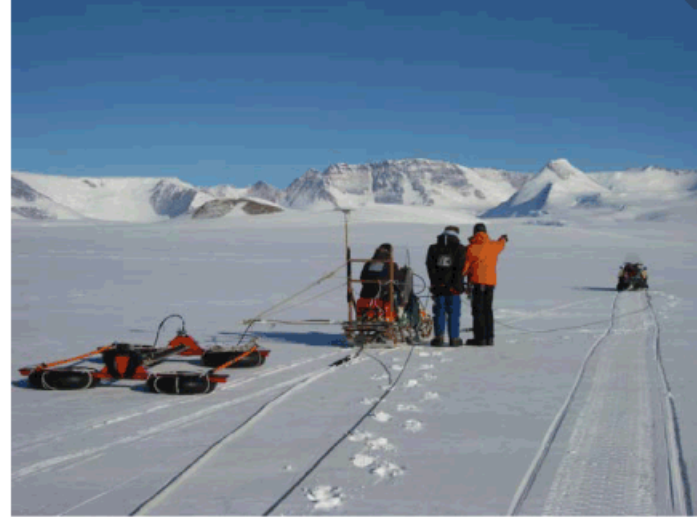
Fig.7: Photo showing Nansen sledge carrying GPR and crevasse rescue equipment
