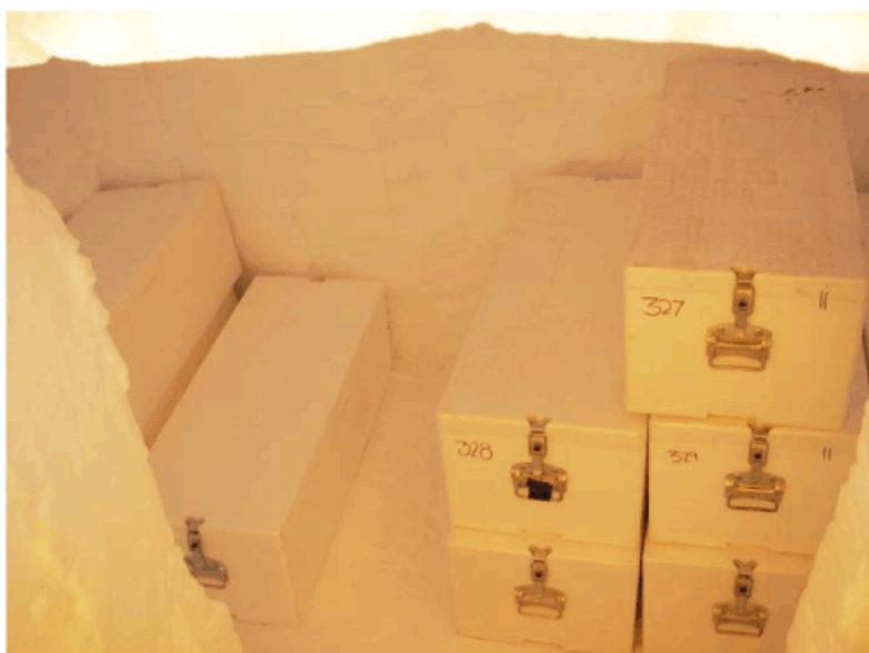
Fig.10: Ice core storage in the field in ice caves cut from the drilling trench
