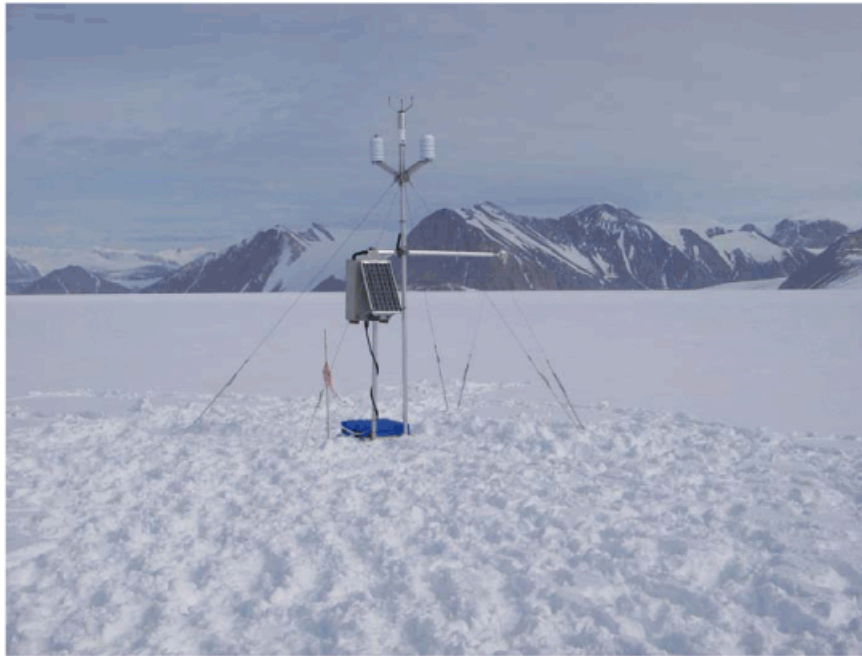
Fig.11: Automatic weather station after the system was dug out and placed a few meters to the south of the original site
