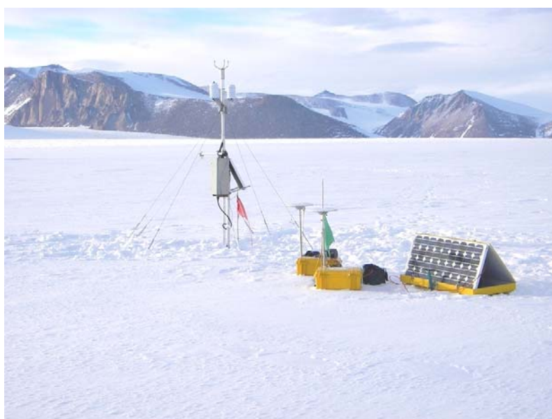
Fig.2: Automatic weather station and submergence velocity devices at Evans Piedmont Glacier
