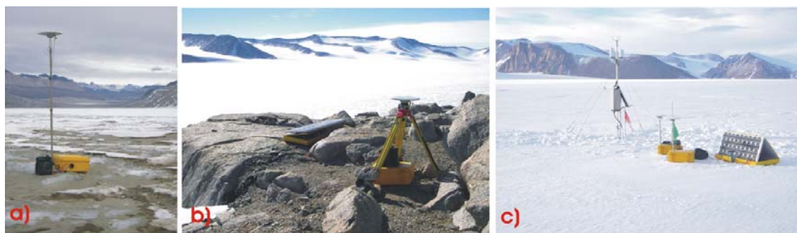
Fig.4: a) submergence velocity device at VLG II (glacier tongue), b) temporary GPS base station at Staeffler Ridge, c) submergence velocity devices at EPG.
