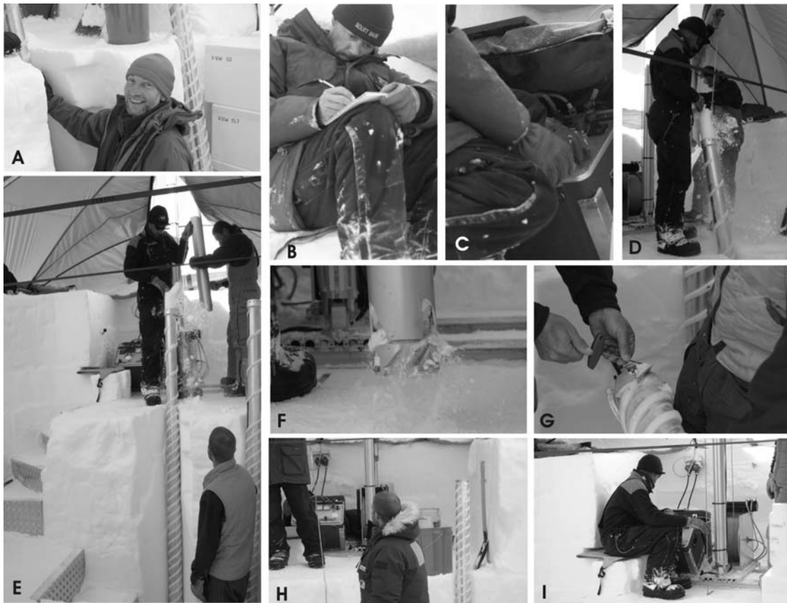
Fig.3: A) Core barrel loading, B) record of core quality, C) control panel, D) extracting cuttings, E) core barrel extracted from drill barrel, F) discharging cuttings, G) adjustment of cutters and core catchers, H) drilling discussions, I) drilling at 165.5m depth.
