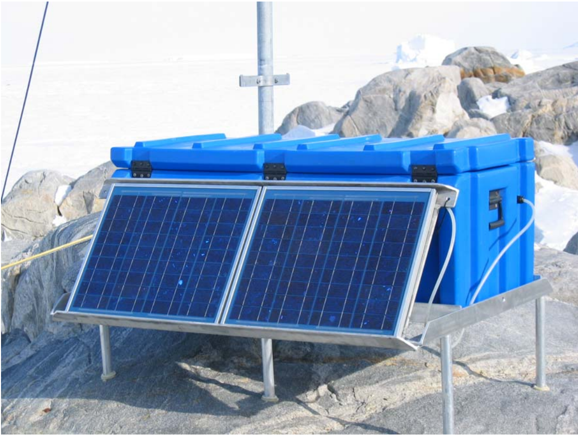
Cape Roberts Tide Gauge Instrumentation. Solar Panel and instruments box. Meteorological mast (background) is not currently in use.
