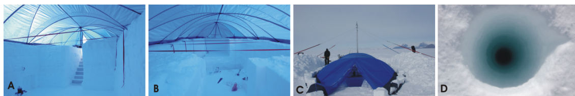
Fig.2 A) and B) inside the drilling tent, C) outside the drilling tent, D) 180m deep borehole
