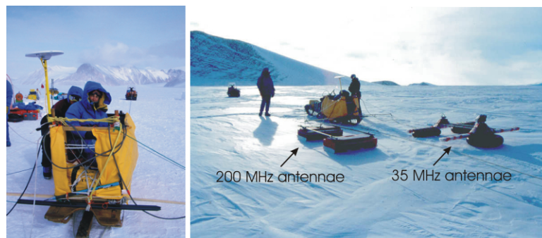
Fig.3: GPR/GPS set-up. A 400MHz antenna travels in front of the first skidoo. A second skidoo tails the set-up for crevasse safety.
