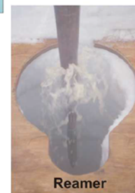
Fig 3. The system uses a combination of melted snow and re-circulated melt-water to produce a jet of hot (95°C) water to melt through the ice shelf. Firstly a vertical pilot hole (~15 cm) is made through the ice shelf. This is then widened to >600 mm using a reamer. Additional reaming is needed at the bottom of the hole as hot water is lost to the ocean beneath the ice shelf.
