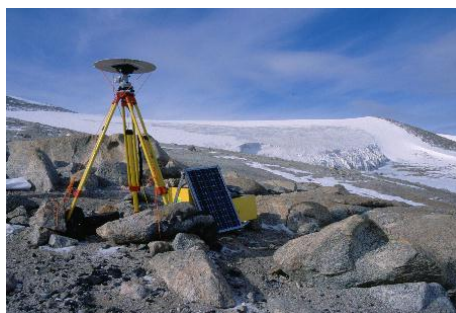
Fig.1 GPS base station
