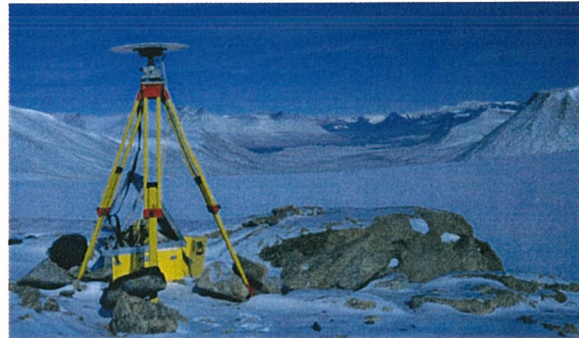
Fig.6: GPS base station
