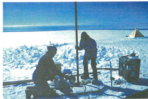
Fig.5: Drilling of firn cores at Wilson Piedmont Glacier
