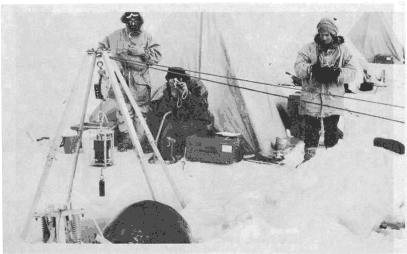
PLATE VI. The current meter ready for lowering as soon as the seal is clear of the hole.
