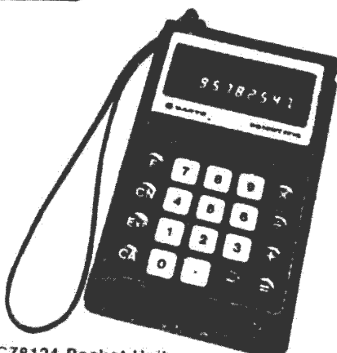
CZ8124 Pocket Unit. A complete 8 digit "economy" scientific calculator with 2 digit exponent. In addition to its basic functions, it has a fully addressable memory, exponents, log, pi, 1/X, V, ex, sin, cos, tan, sin -1 , cos -1 , tan -1 , radians and degrees. AC or DC power. $80.50 without AC adaptor.
